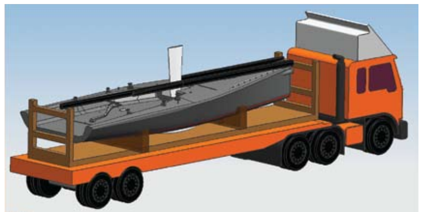
Horizontal keel retracted on flatrack
